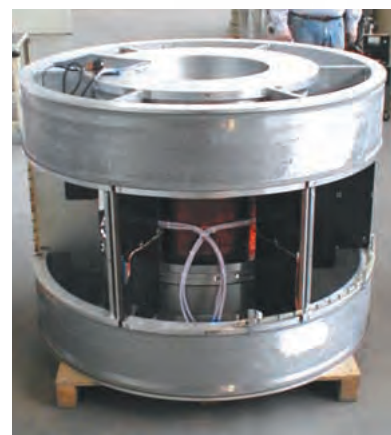
Actively shielded magnet system (left) and magnet coil (right) of the BioSpec® 47/40 USR
